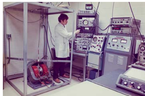
Heyman performs an ultrasonic test on a semiconductor in a magnetic field to assess the coupling between charge carriers and phonon waves. Photo Courtesy of Joseph Heyman
