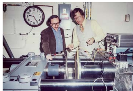
Heyman (right) explains his idea for using a sonic wave to test the adhesion of Shuttle tiles in 1981. Courtesy photo
