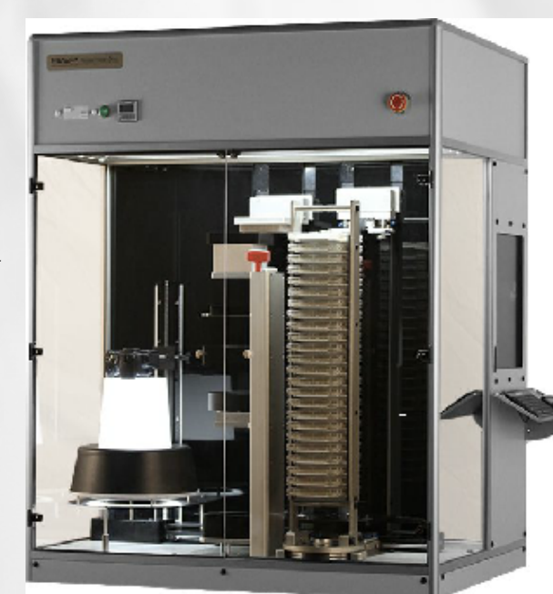
Figure 2. BM3-BC Colony Processing Robot Automated colony picking between selective media
